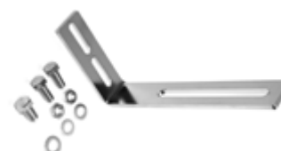
TC1279-183KIT Mounting bracket kit, heavy duty, wall & strut This kit has two vertical slots suited to wall or Unistrut™ mounting and provides a single long slot to accept duct mounting brackets up to 220mm size. Note: Individual duct "C" type brackets are required in addition to this kit (see mounting hardware).
