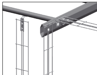
B30-I mounted onto cable ladder.
