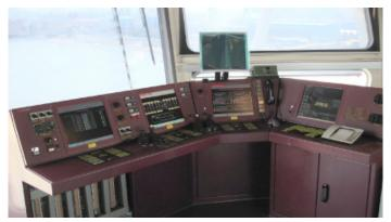
The second problem is the small amount of production: only five monitors are needed. Moreover, the custom design involves not only the implementation of the larger monitors, but also the demand for deep dimming backlight and ARcoated high contrast glass.
